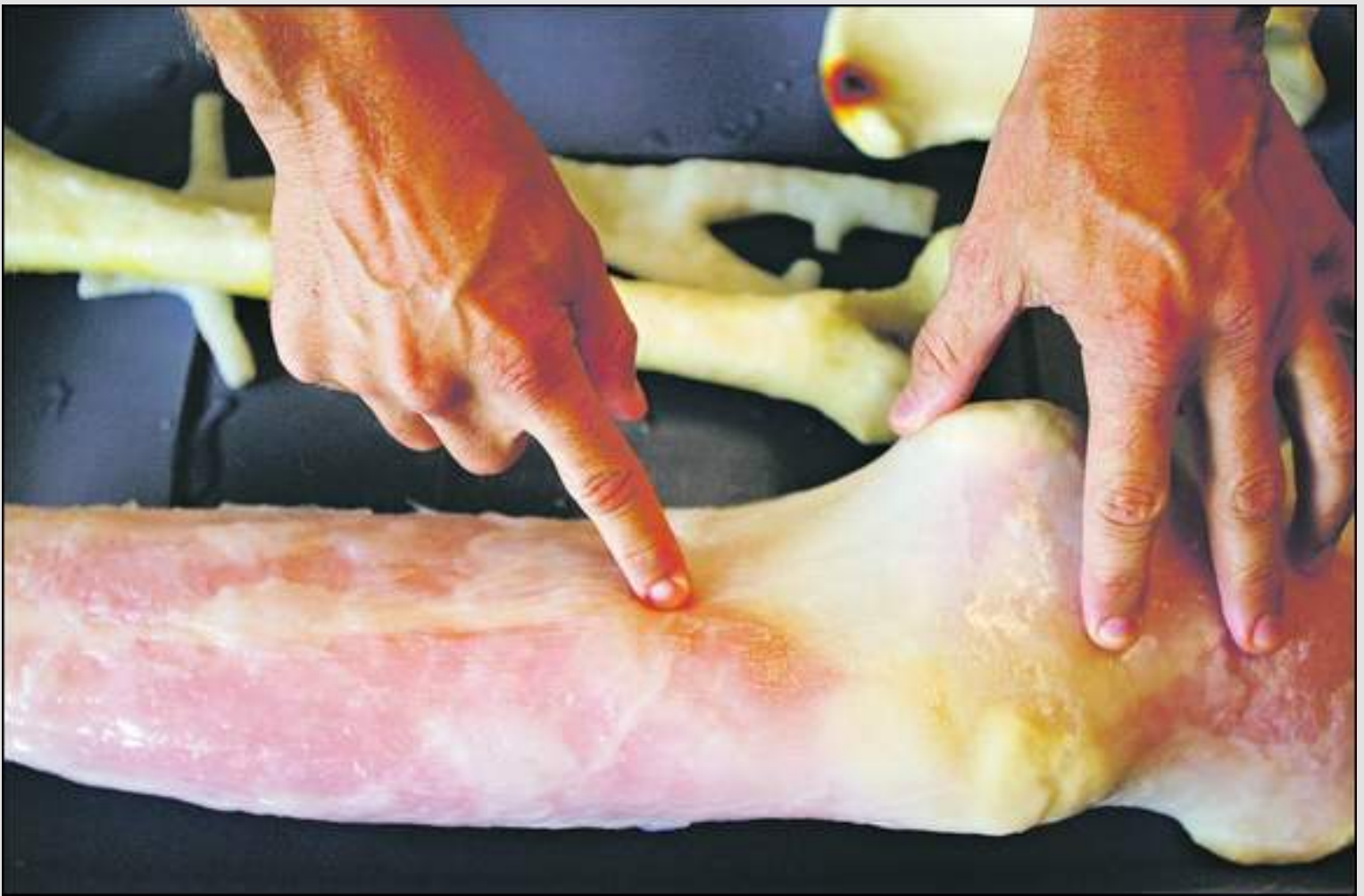
Dr. Christopher Sakezles, President and Chief Technology Officer of SynDaver Labs, shows a synthetic human thigh made by his company to replace live animals in medical device development tests.
